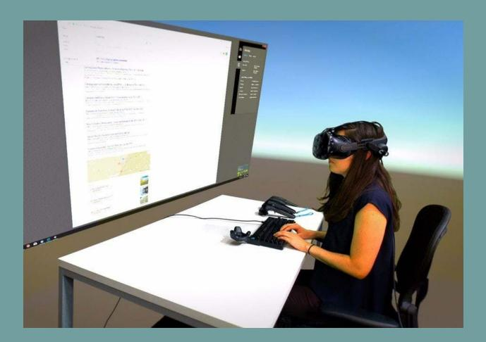
The HTC Vive Tracker is represented as a keyboard (precisely overlaid virtual 3D model) across the Steam VR system, and contains animations for key presses. It is compatible with all apps using SteamVR as their building block, and the keyboard overlay appears automatically as soon as the Vive Tracker is turned on. It uses the existing downward facing camera on the Vive VR headset to render your hands in VR.
